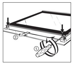
Loosen the screws with a Torx screwdriver then remove the guides and the trim with the seal.
